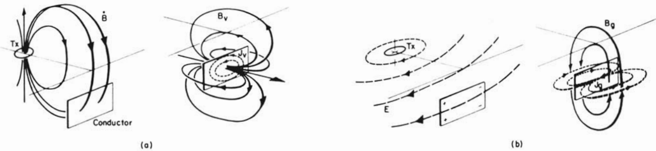
FIG. 1. EM fields and currents about a conductive plate in a conductive half-space. Solid lines indicate magnetic field components, dashed lines indicate electric field components and currents. (a) Illustrates the generation of vortex currents J_v by inductive coupling with the component of d\mathbf{B}/dt normal to the plane of the plate. B_v is the secondary magnetic field due to the vortex currents. (b) Illustrates the generation of channeled currents J_g by galvanic coupling with the component of the primary electric field \mathbf{E} in the plane of the plate. B_g is the secondary magnetic field due to the galvanic current.
