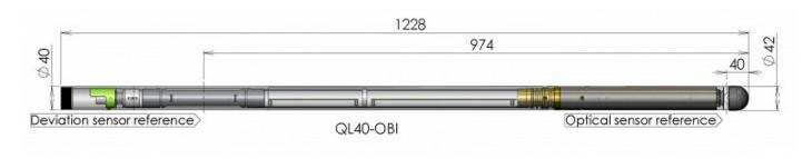
Schematic drawing of QL40-OBI. Image courtesy of Mount Sopris Instruments.
