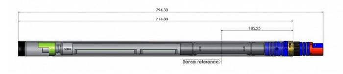
Schematic drawing of QL40-DEV. Image courtesy of Mount Sopris Instruments.
