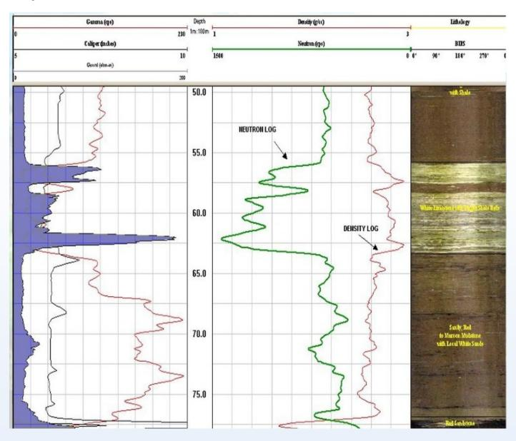
This tool enables the user to obtain real time quantitative porosity measurements in wet, dry and muddy conditions, whilst improving the imaging resolution, allowing the user to image thin lithological beds. As this is a quick Link bottom sub, the QL40-NEU can be stacked with the other QL tools in the product line, allowing more versatility and
