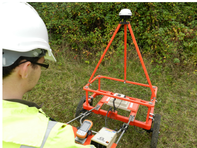
EM61MK2 set-up for typical brown field site.
