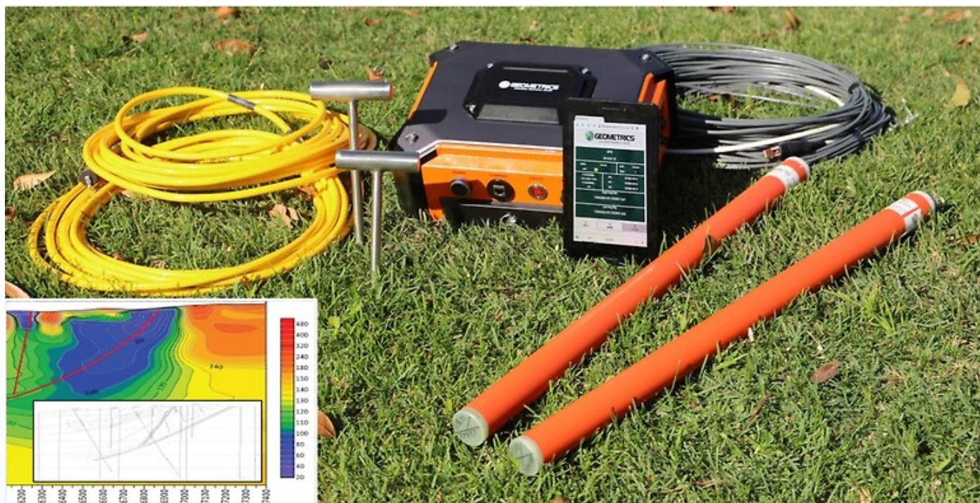
Fig. 1. Shows the Stratagem EH-5 components which includes the Stratagem console, Android tablet, stakes, cables and mag coils. The image on the left is a 2D inverted dataset from a mineral exploration study using the EH-5 showing a 65°-75° striking fault, close correlation to the geological map of the area (Image Courteously provided by Geometrics Inc)
