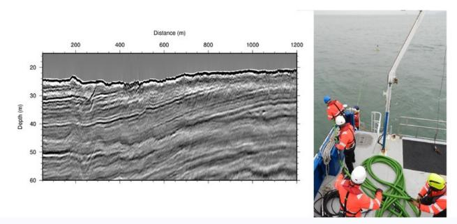
In addition to the higher 16kHz sample rate the GeoEel LH-16 also boast a much higher data transfer rate to allow for up to quarter second shot intervals (with a 48 channel array) with sparker and boomer sources.
