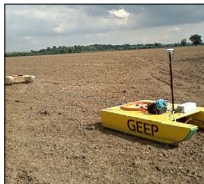
GEEP with subsidiary deck for EM34 survey
