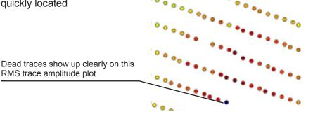
Different sized elements show which shots are completed and which geophones can be picked up
