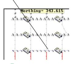
Map View color coding highlights receiver positions needed for any shot but not yet installed
