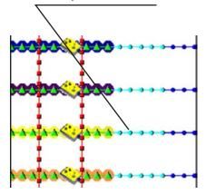
Geometry parameters like line number, distance from next shot, and trace number can be color coded to look for errors and inconsistencies
