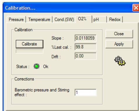
**Figure 5-4** Oxygen calibration
