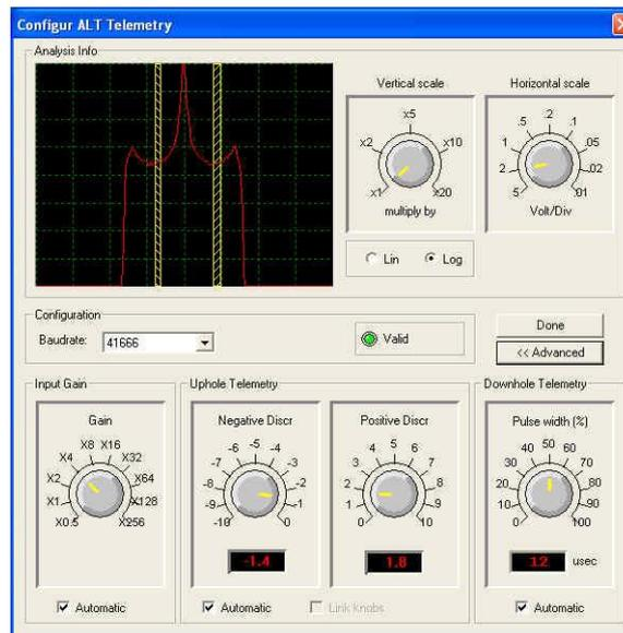
*Figure 4-7 Matrix telemetry settings*
