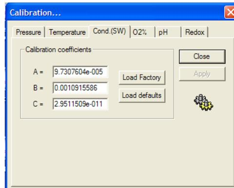
**Figure 5-3** Conductivity calibration
