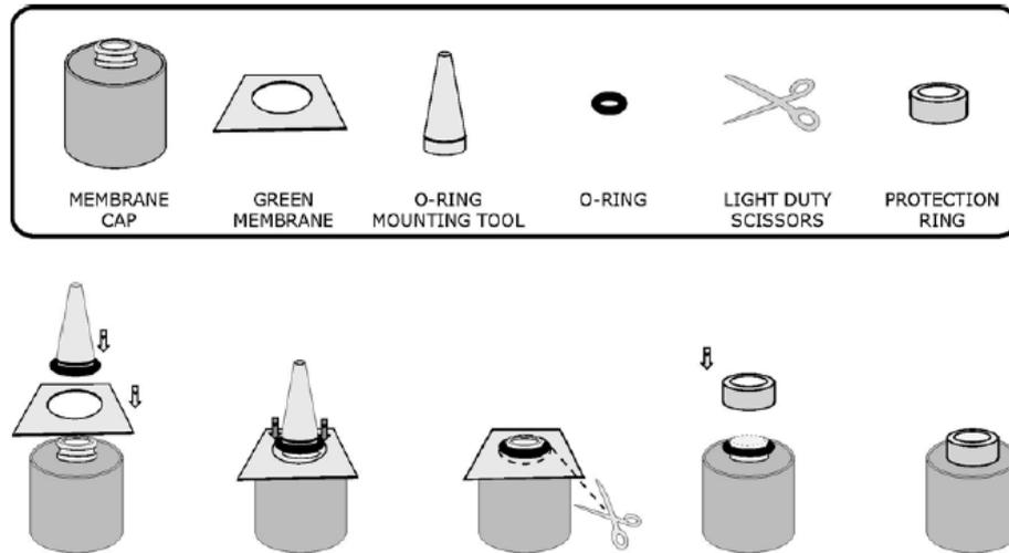
**Figure 6-1** Oxygen sensor maintenance kit
