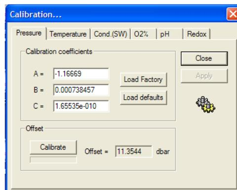
**Figure 5-1** Pressure sensor calibration
