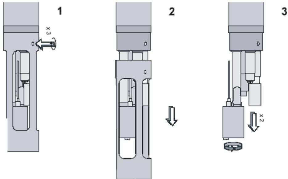
**Figure 4-5** Dismounting the sensor protection cage
