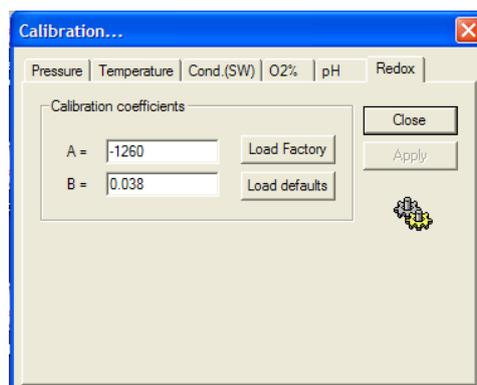
**Figure 5-6** Redox calibration
