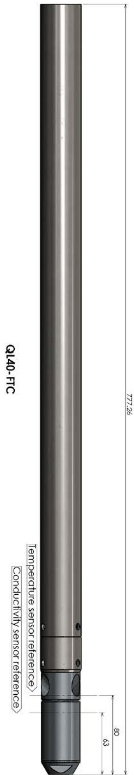
Figure 1-1 QL40 FTC Dimensions (bottom sub)
