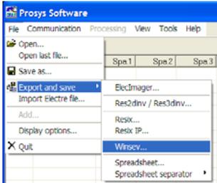
**Second step:** Always with the PROSYS software, create a file at the format of the WINSEV inversion software, using 'file, export and save, Winsev' instructions and give a name to this new file: **test.ws3**
