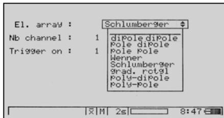
**"El array"** function for selecting the electrode array (Schlumberger)
