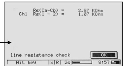
Then, the ground resistances of the electrodes are checked ( $R_{AB}$  and  $R_{MN}$ )
