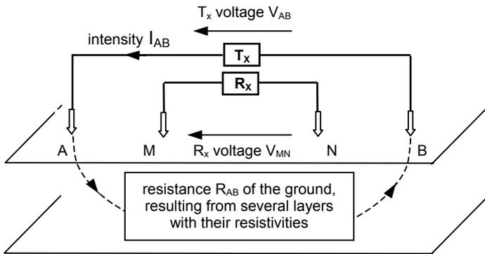
$$INTENSITY = Tx \text{ voltage} / \text{resistance}$$
