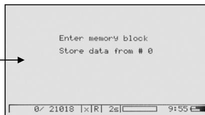
Storage of the measurement; confirm the memory location (0 to 21 000)
