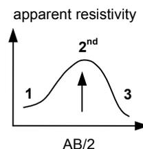
If a **thin 2<sup>nd</sup> layer is more resistive** than the two other ones, it is the product thickness x resistivity (known as the transverse resistance) which is invariant: a 30m thick 20 ohm.m second layer gives the same apparent resistivity curve as a 15m thick 40 ohm.m layer (resistance 600 ohm.m<sup>2</sup>).
