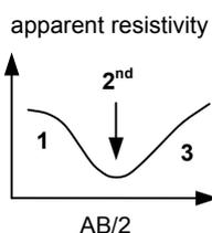
In case of a 3 layer ground, if a **thin 2<sup>nd</sup> layer is less resistive** than the two other ones, only the ratio thickness / resistivity (known as the longitudinal conductance) characterizes this second layer: a 30m thick 20 ohm.m second layer gives the same apparent resistivity curve as a 15m thick 10 ohm.m layer (conductance 1.5 S)
