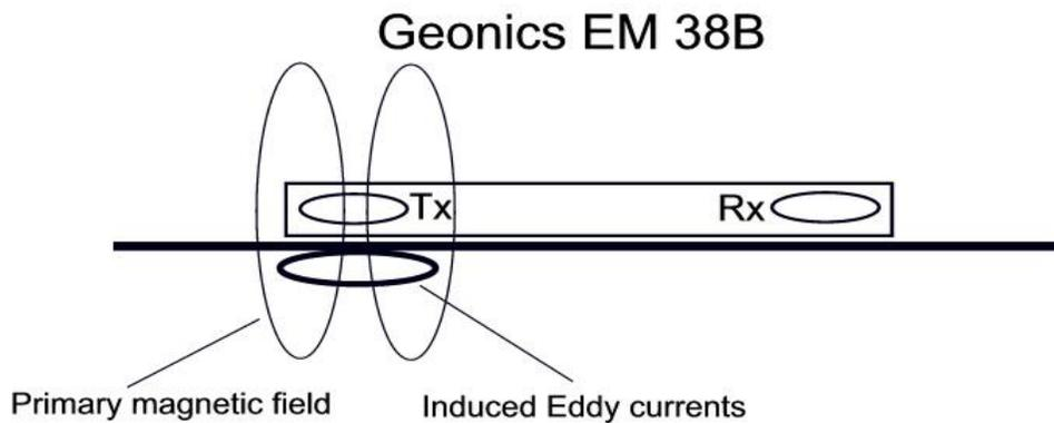
In all of these instruments a small transmitter coil is energized with an alternating current at an audio frequency. This current generates, in turn, an alternating primary magnetic field in the ground, as shown in the figure. The time-varying magnetic field causes two important effects.
