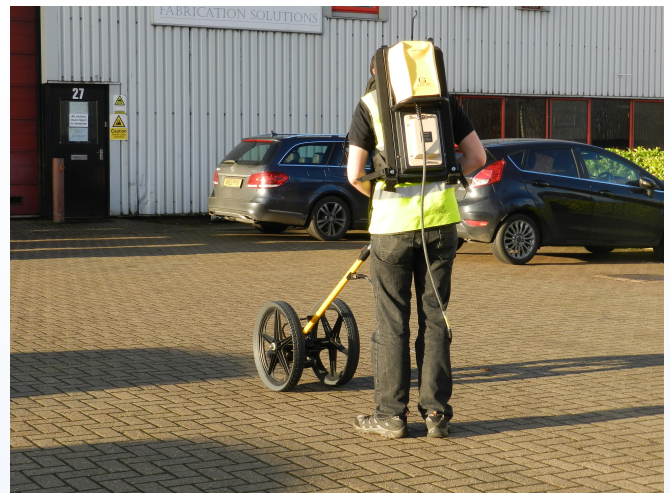
EM61HH MK2 surveying urban site.
