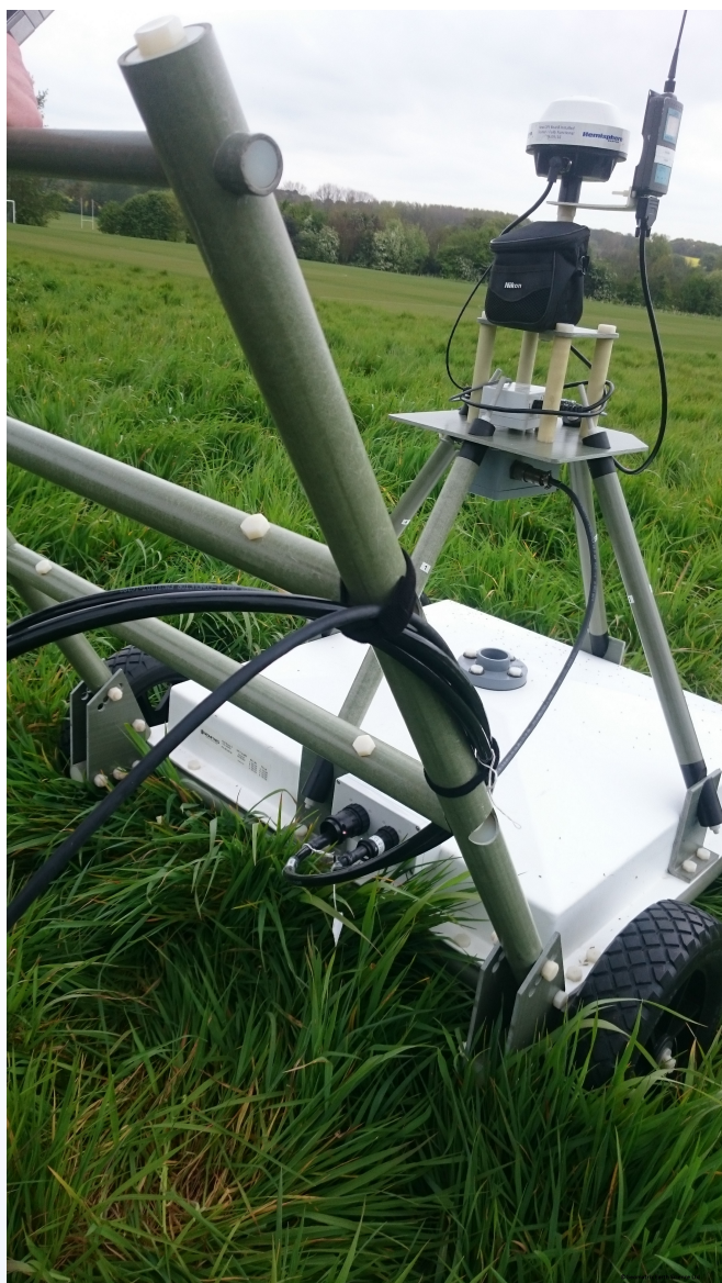
Picture of the MetalMapper2x2 in action at the NSGG test site locating buried mock UXO targets.
