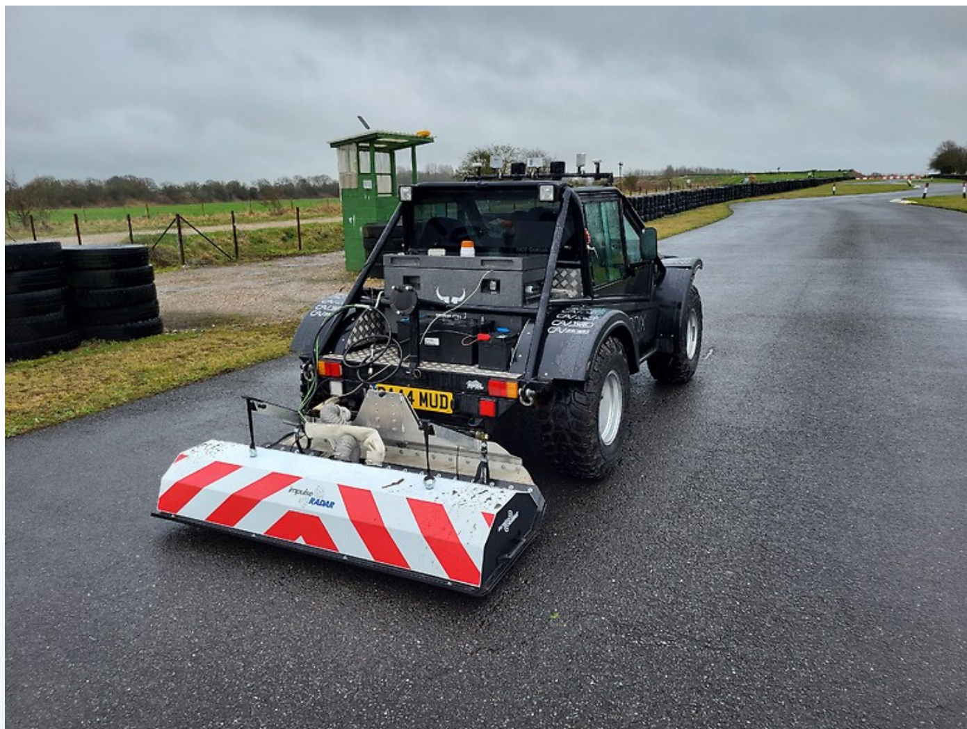
Fig 1. Shows the features of the vehicle carrier and how it fixes onto a survey vehicle (Image courteously provided by impulse radar)
