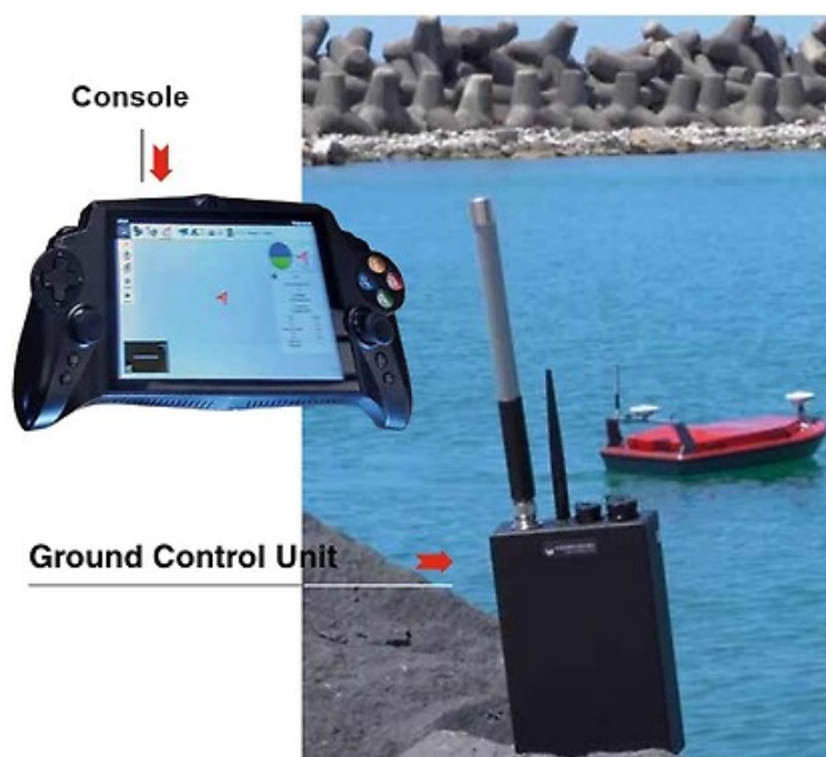
Fig. 3. Sestante autopilot system designed by Codevintec, image shows the ground control unit which fits to the ATV and the smart controller which is used by the operator to control the system, image courteously provided by Codevintec Srl
