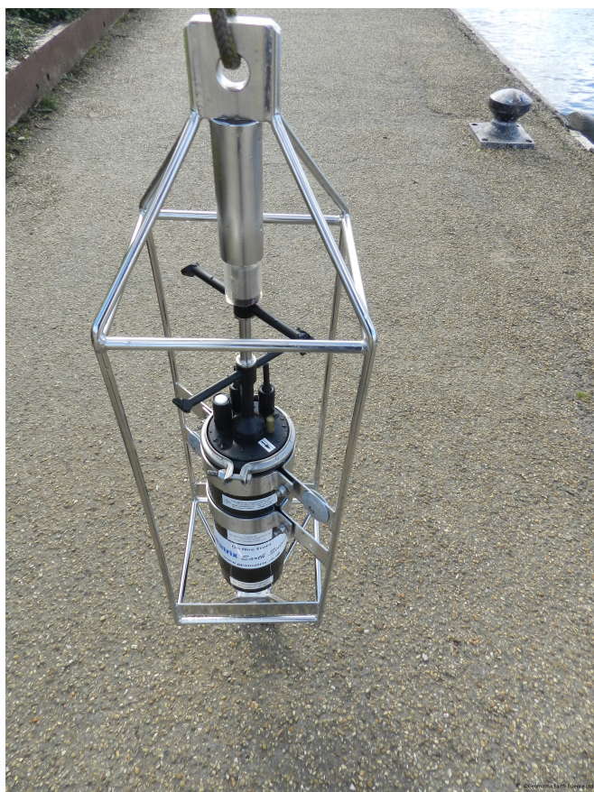
ACM Wave Plus look at CTD and auxiliary port bulk head.
