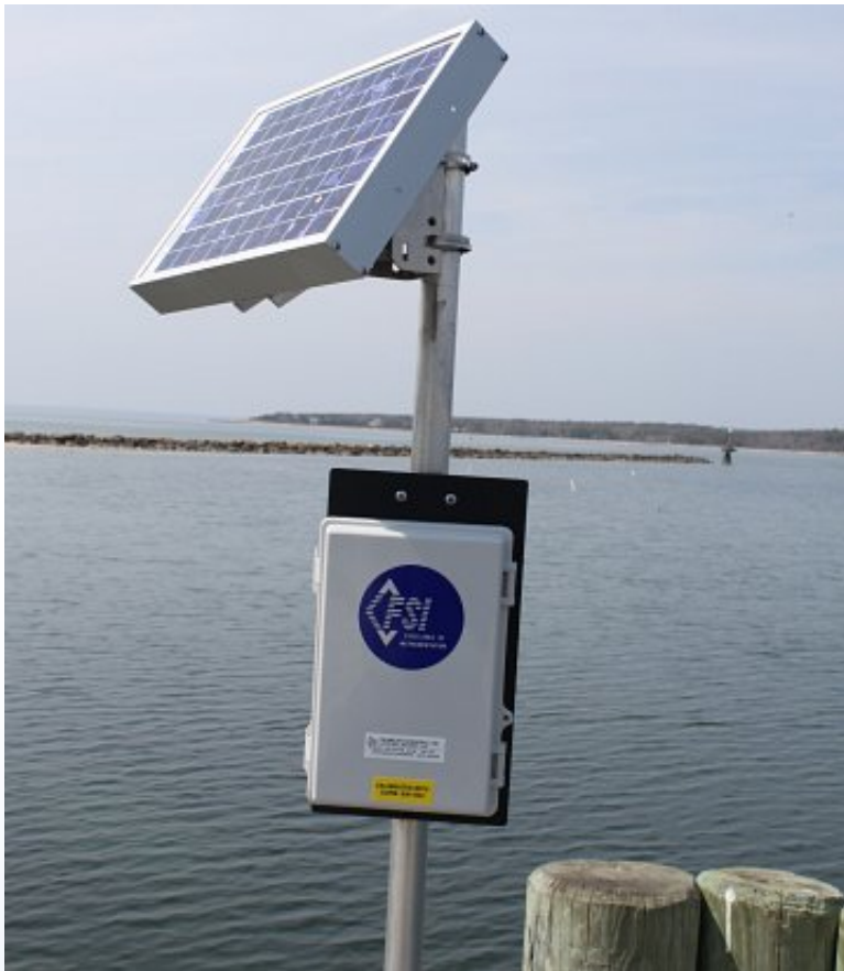
Tide Monitoring system deployment with solar panel. Image courtesy of Falmouth Scientific Inc.
