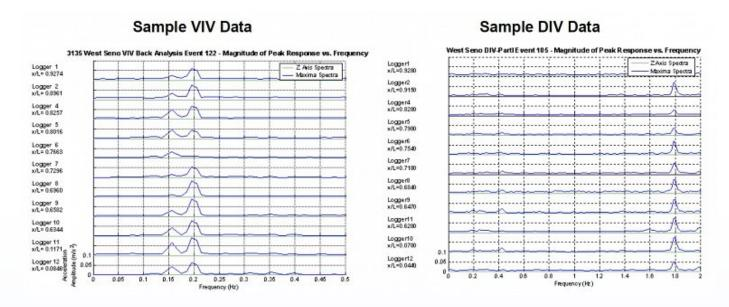
Example Vortex Induced Vibration (VIV) and Drilling Induced Vibrations (DIV) events. Courtesy of Falmouth Scientific Inc.
