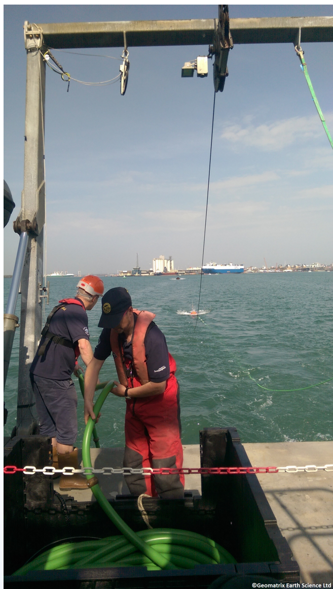
Hand deployment of the MicroEel off of the back deck.
