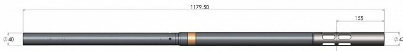
QL40-OCEAN water sampling probe schematic. Image courtesy of Mt Sopris Instruments.
