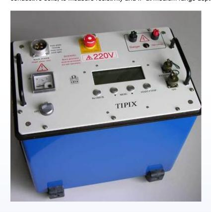
With the possibility to limit current, power, voltage, and the different self-test and quality control of the injected signal, the TIPIX ensure a good protection for the device and he operator. This instruments features 4 buttons on the front face that allow the operator to select manually different voltage injection levels. The "automatic range" mode allow to select automatically the optimal injection level regarding the contact resistance.
