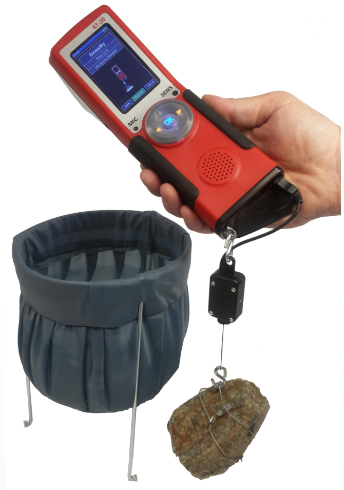
KT20 density measurement- first the sample is weighed in air. Image courtesy of Terraplus..
