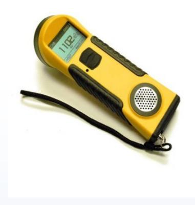
Although the KT10H includes the sample pin and automatic measurement function for rough surfaces this meter performs best on processed samples with even volume and smooth surface to exploit the sensor sensitivity.
