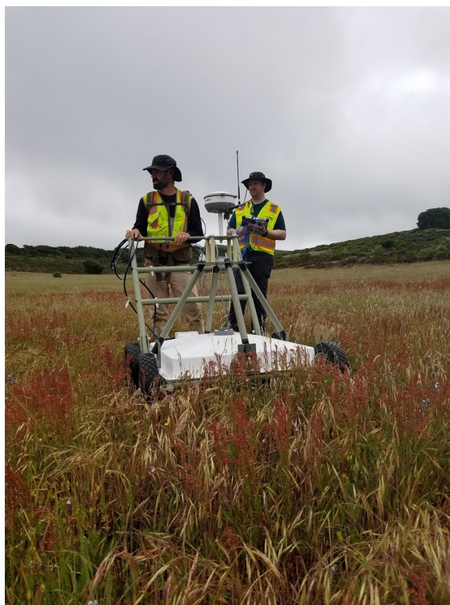
MetalMapper2x2 undertaking a prove-out at Ft. Ord, in Seaside, CA. Ordnance Detection and Discrimination System (ODDS) plot.
