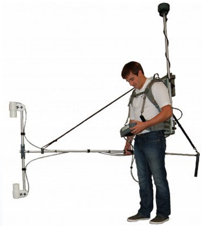
Geometrics G-858 Gradiometer & GPS setup
