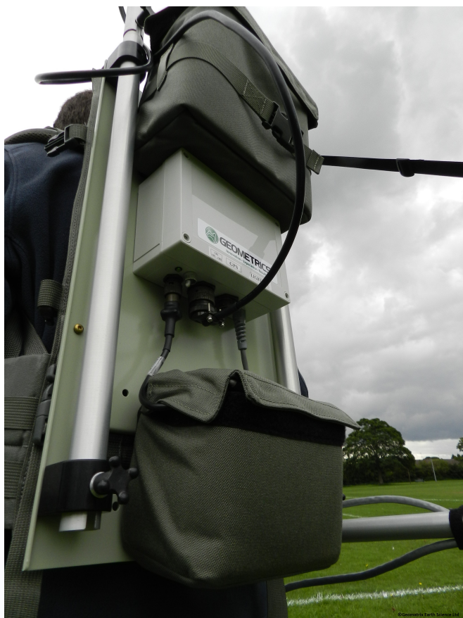
G-858 Backpack, showing battery pouch.
