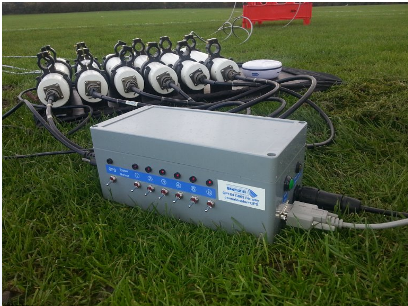
The Geomatrix Six Way Concatenator with English Heritage's 6 G-862 Cs magnetometers.
