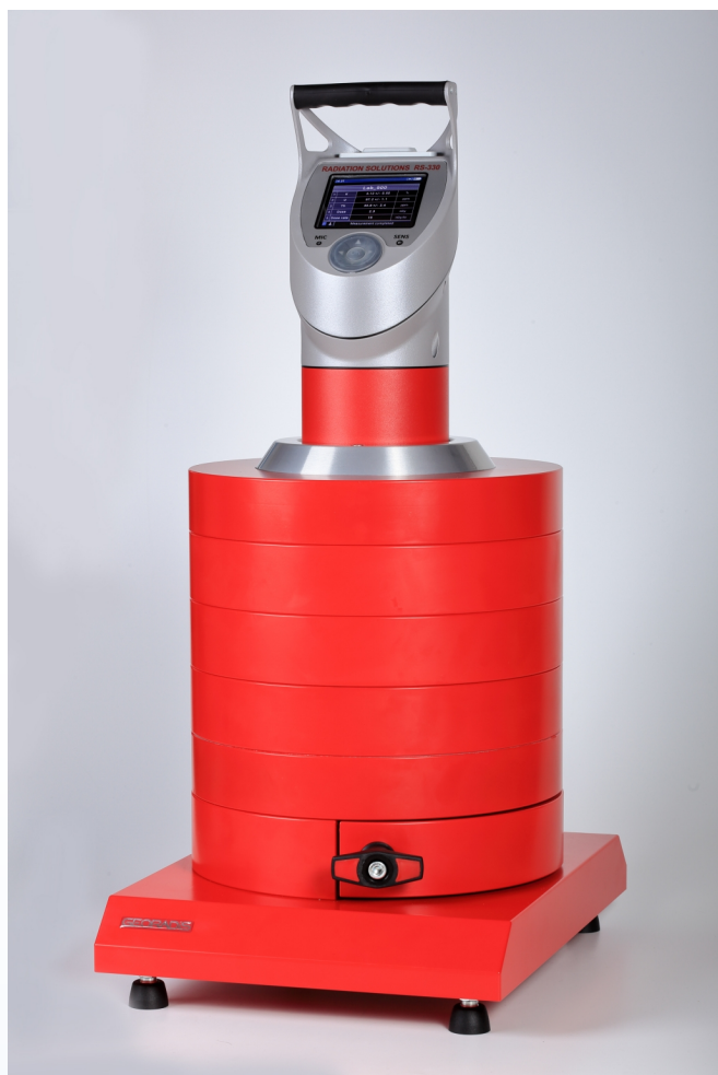
The GT40 Laboratory stand with Lead shielding and sample chamber.
