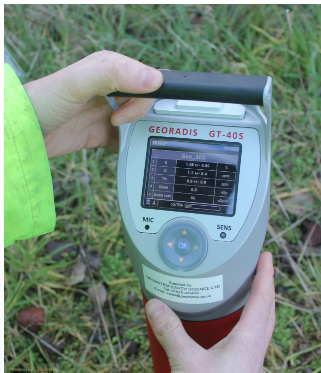
GT40 offers a simple GUI and daylight visible screen.
