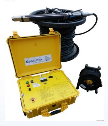
The borehole source is coupled to the borehole wall by a pneumatic clamping system (inflatable bladder). The orientation of the source is controlled from surface by a torsionally stiff hose.
