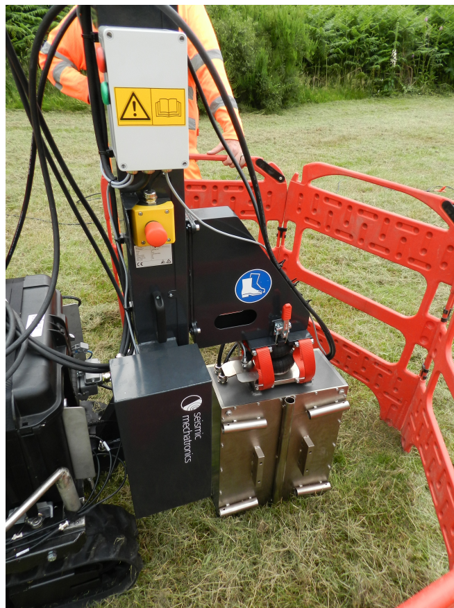
Lightning setup for a P-wave sweep.
