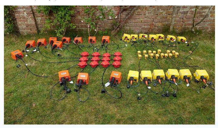
The Atom's primarily application is low frequency passive wave data acquisition. Typically 11 to 100 of units are deployed over a large area and record independently for multiple days. As each Atom is a complete recording device the operator is not constrained by cables or a laptop/data logger, and can deploy non-uniform arrays.
