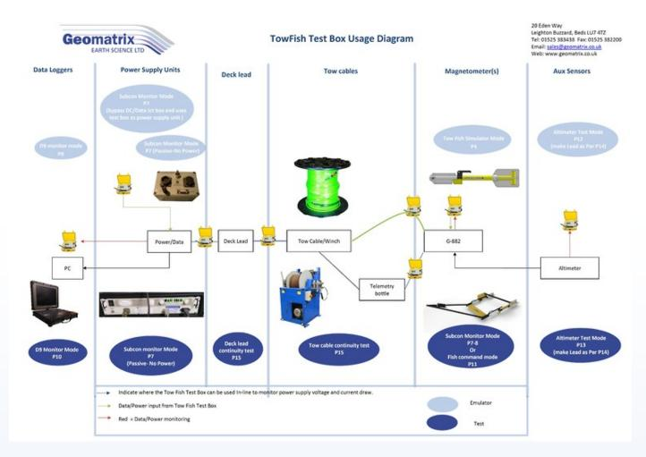
This diagram illustrates when and how the Tow Fish Test Box can be used to test various G-882 marine magnetometer system components.
