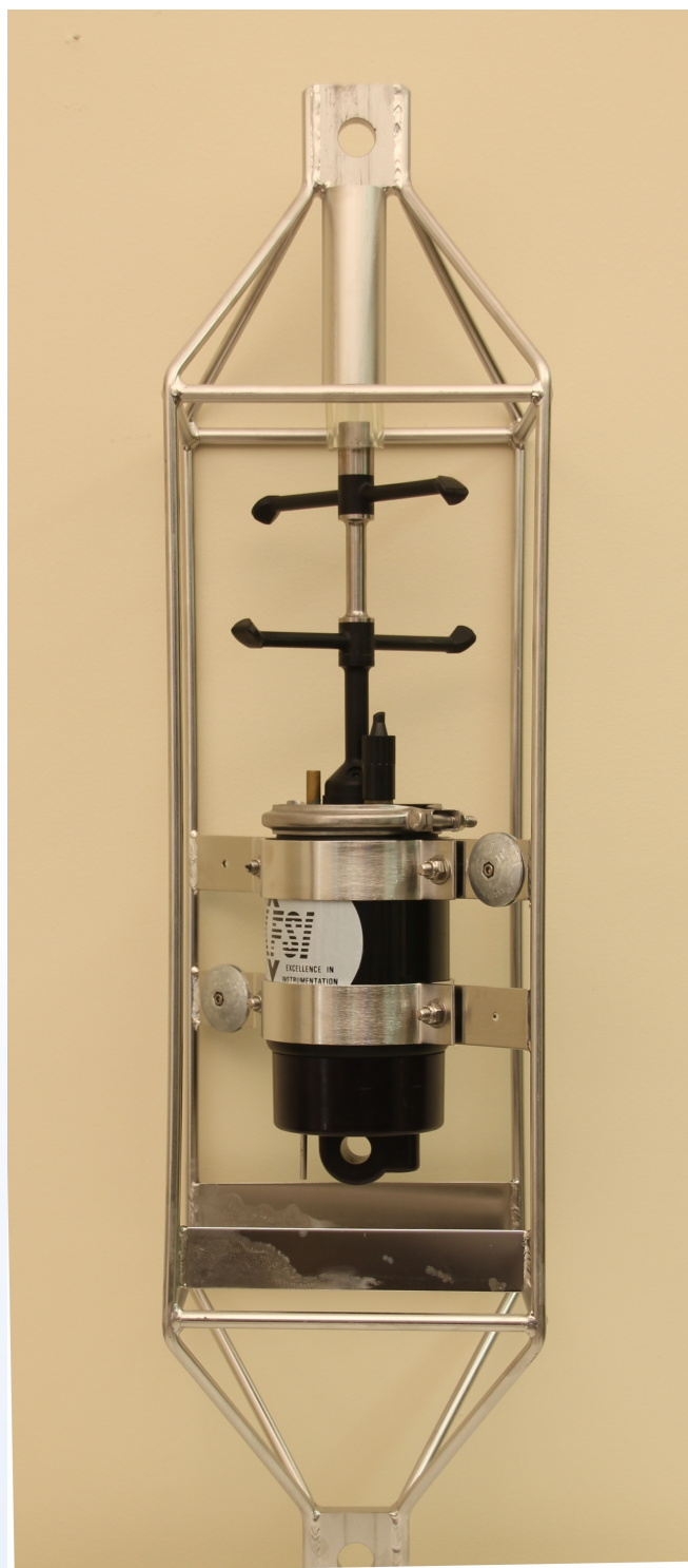
ACM-PLUS with 200m epoxy housing and 5 Ton mooring frame and CTD.
