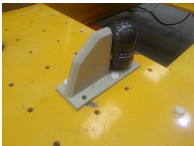
Tritech iGC mounted on the GEEP multi sensor platform.
