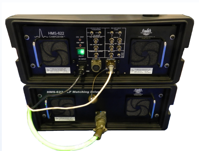
Top end power supply and Analogue A/D electronics module. The secondary module is only required for Low Frequency and Ultra Low Frequency transducers.
