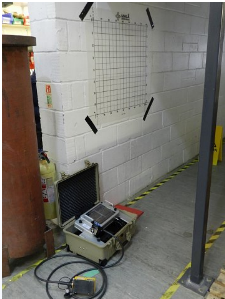
CX12 being used to identify any cavities behind a breeze block wall.
