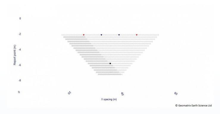
The software enables the user to configure bespoke 2D or 3D measurement routines, using one or more quadrupole configurations, upload them to the instrument and schedule a time for data acquisition is to commence. Results can then be viewed in real time in a number of forms to aid quality control or evaluated after the sequence has been completed.
