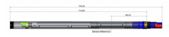
Schematic drawing of QL40-DEV. Image courtesy of Mount Sopris Instruments.
