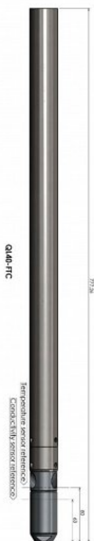
QL40-FTC Schematic. Image courtesy of Mount Sopris Instruments.
