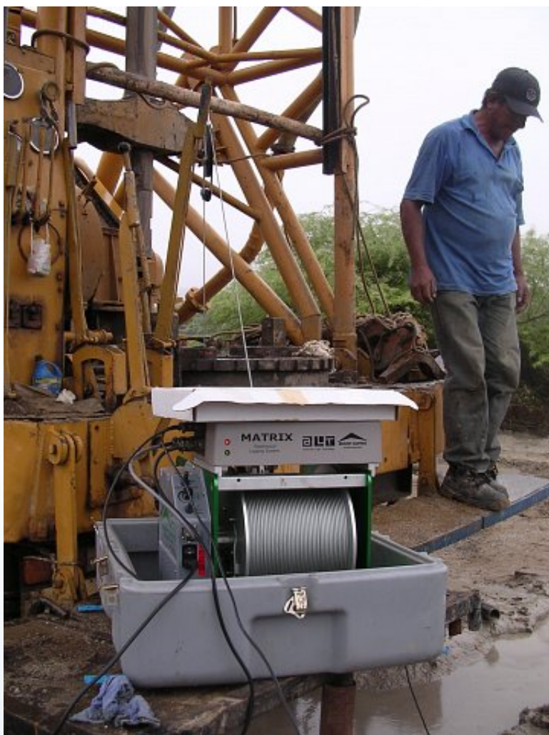
MX Winch deployment off of a Drill Rig. Image courtesy of Mount Sopris Instruments.
