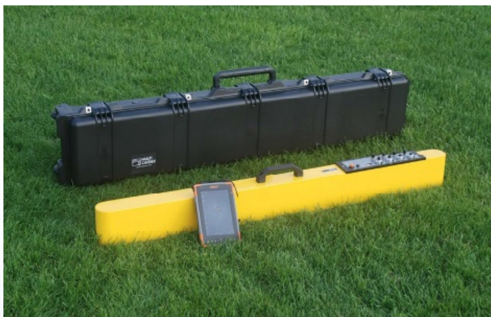
Fig 1. Image of the EM38mk2, including case and an example datalogger you can use with the instrument, Image courteously provided by Geonics Inc
