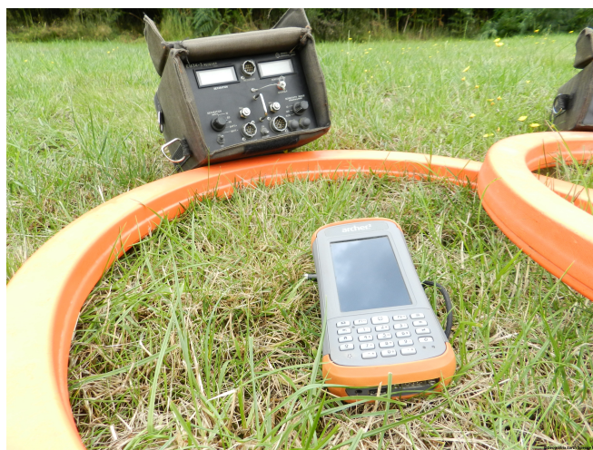
EM34-3 close up of Receiver
