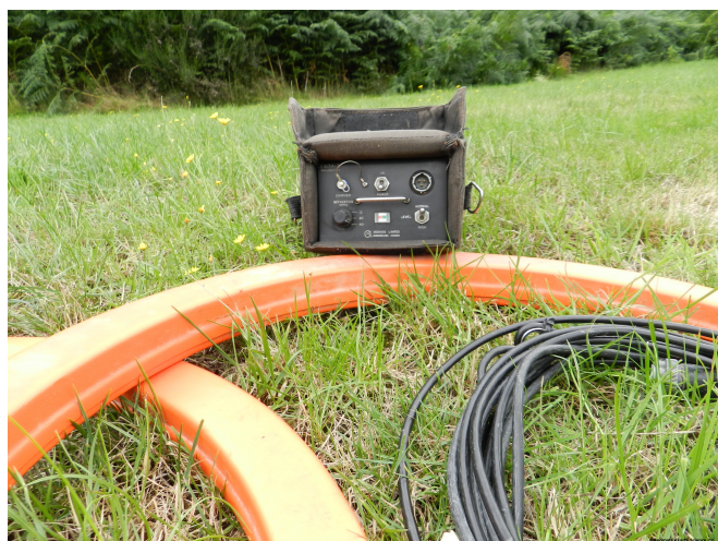
EM34-3 close up of Transmitter
