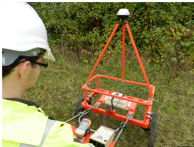
EM61MK2 set-up for typical brown field site.
