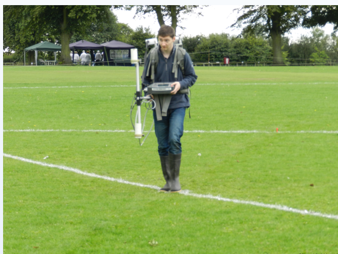
Jonathan undertaking a Heading Error test
