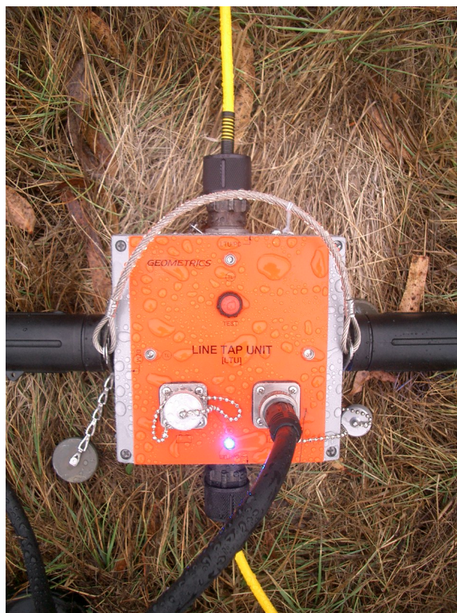
GeodeDZ central line tap unit, used to pass data from each line back to the recording console.
