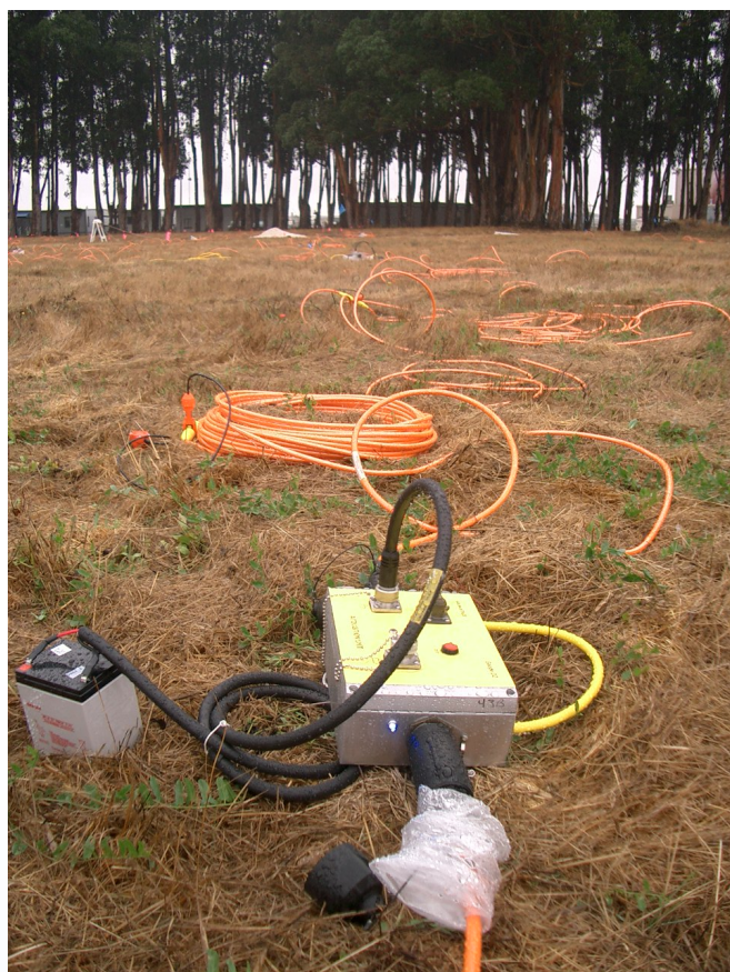
GeodeDZ Seismograph and spread cable
