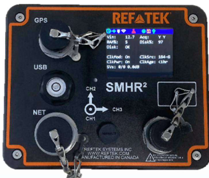
Fig 1 - Image of the SMHR 2 Integrated Seismic Recorder and Accelerometer depicting the ports and data screen, includes 3 adjustable feet for levelling. (Image courteously provided by Reftek)
