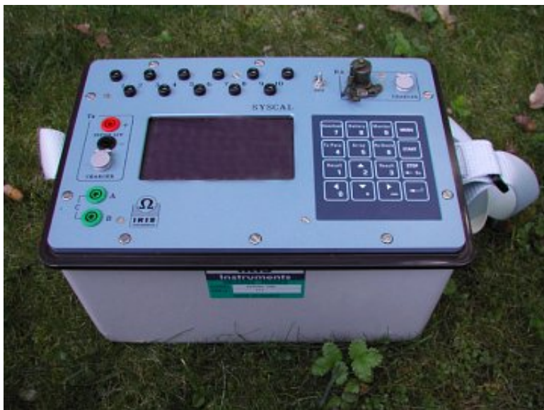
Syscal Pro Deep Marine console (image courtesy of Iris Instruments)
