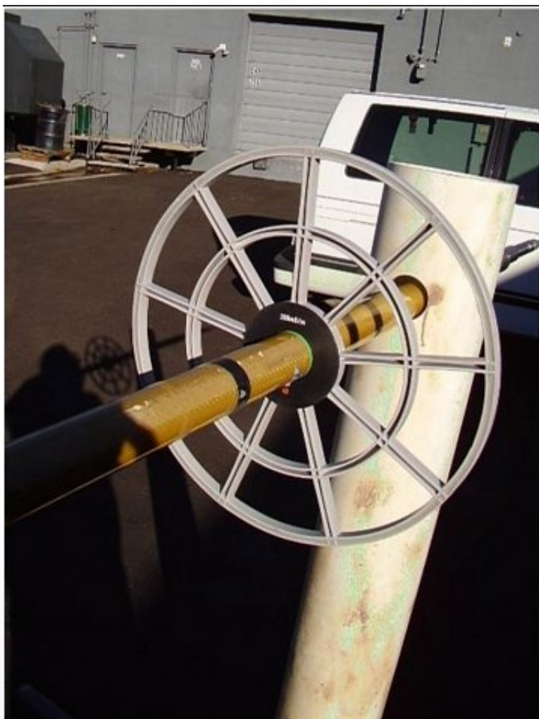
QL40-IND fitted with calibration coil. Image courtesy of Mt Sopris Instruments.
