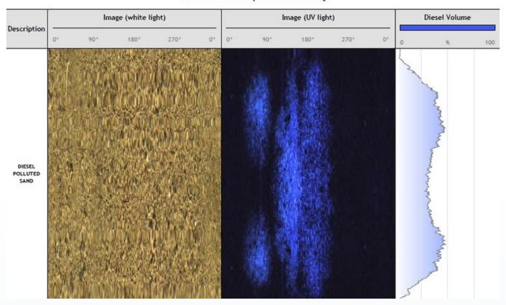
The QL40-OBI2G-UV probe was utilized in a pollution study to analyze diesel fuel concentrations within a silica-rich sand body. Image supplied by Mt Sopris.
