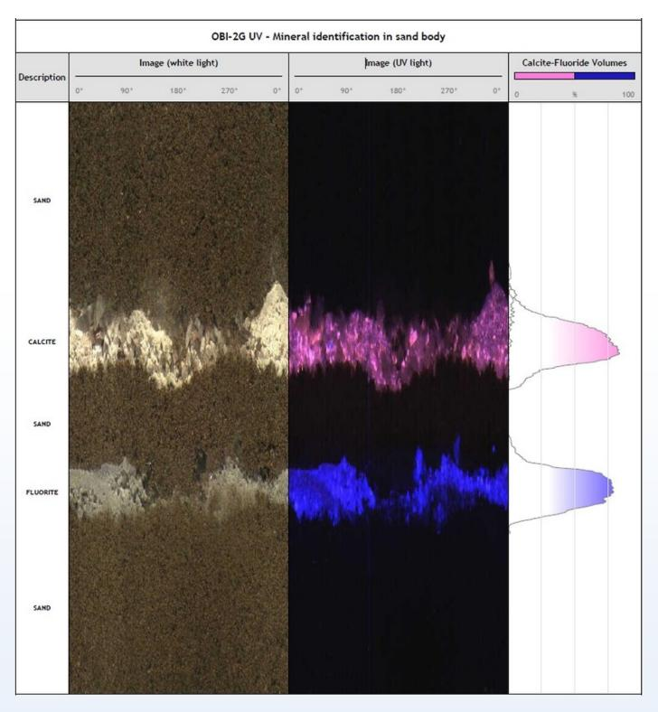
The QL40-OBI2G-UV probe was deployed in a study to analyze the concentrations of calcite and fluorite minerals within a silica-rich sand body Image supplied by Mt Sopris.
